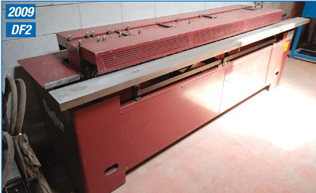
2009 FLAGLER Duct Flange Machine, Model DF2, 35-300, 14 Station, 18-26 Gauge Capacity, 60 FPM, 7.5 HP, 575V, sn DF2-151-1209
