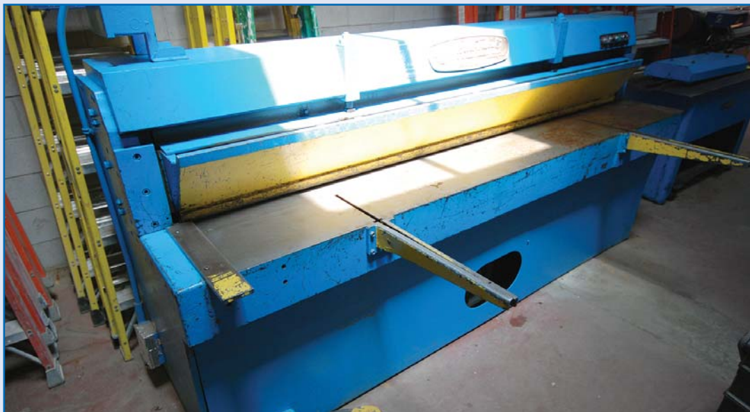
EDWARDS 8' x 1/8" (125G) Power Shear, Foot Pedal Control, 2 Material Supports, sn 892679
